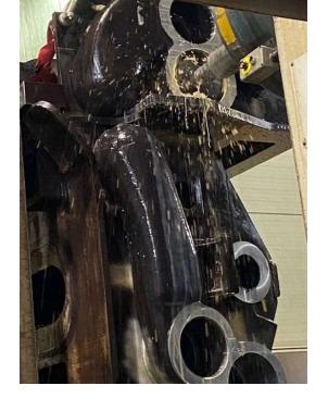
To date, the components for the P2's cylinder block have been cut and formed, the fabrication has been welded together and stress-relieved and machining is well underway. In October, the monobloc took a short break from the machining work to visit DLW for the convention, but machining will continue on return to Howco in Irvine.
